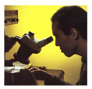
autoclave. The sensors communicate data to the system's computer about the chemical changes occurring. At left below, Micromet's Dr. Huan Lee is preparing a test of a polymer resin, dipping a ribbon sensor in the resin; the large black box is the Eumetric System II Microdielectrometer. Above, Lee is using a microscope to position the silicon microchip on the ribbon and at center right engineers are studying the results of the test.
