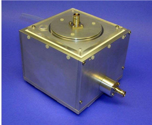
Figure 1 LT-4123 Liquid Dielectric Test Cell
