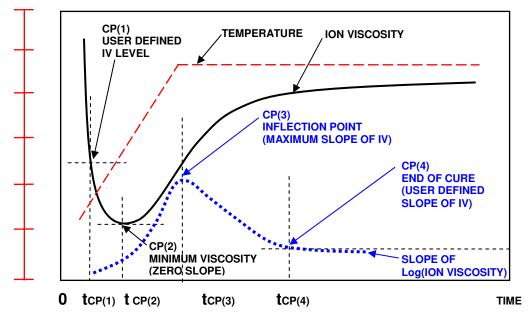
Figure 25-3 Ion viscosity curve and slope of ion viscosity of a curing thermoset
