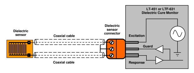
Figure 5 Connecting a dielectric sensor using shielded leads
