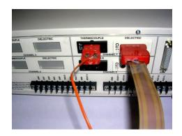
Figure 2 Rear panel of dielectric cure monitor showing dielectric and thermocouple sensor connections
