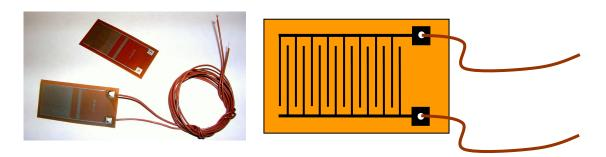
Figure 3 Mini-Varicon sensor and schematic representation
