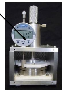
Figure 3 LT-4203 Parallel Plate Test Fixture (Showing "ZERO" button)
