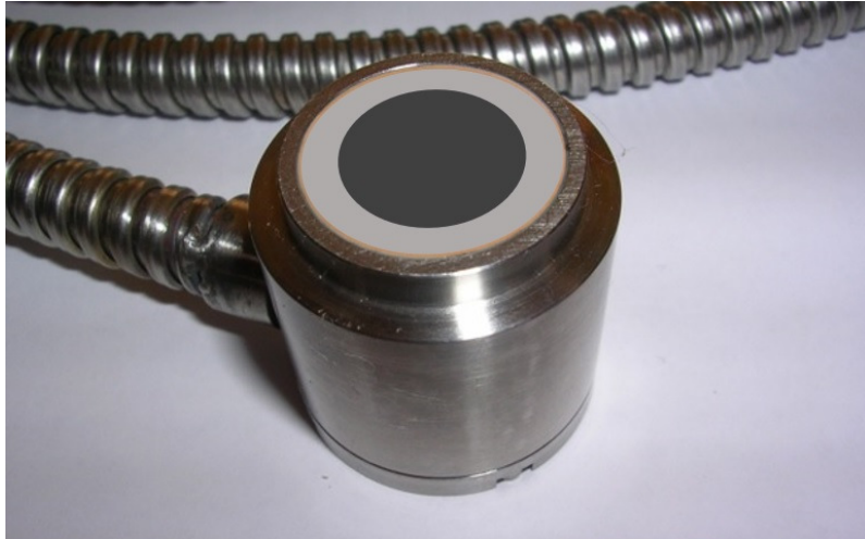
Figure 37-9 Carbon+Unitrode coated, reusable sensor
