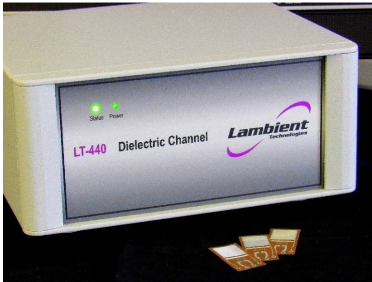
Figure 37-1 LT-440 Dielectric Channel with AC/DC cure monitoring capability
