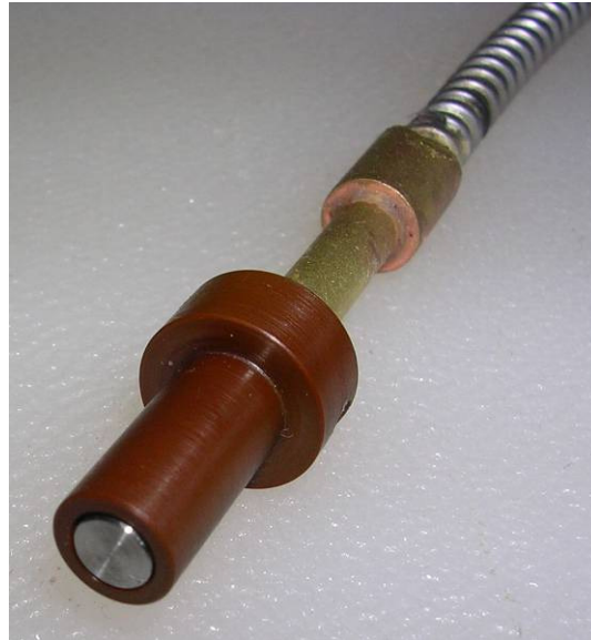
Figure 1 6 mm diameter reusable dielectric/conductivity sensor
