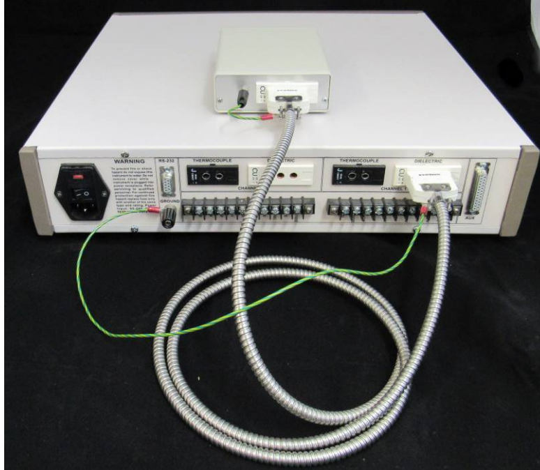
Figure 5 c Cable connections from LT-451 to transition box
