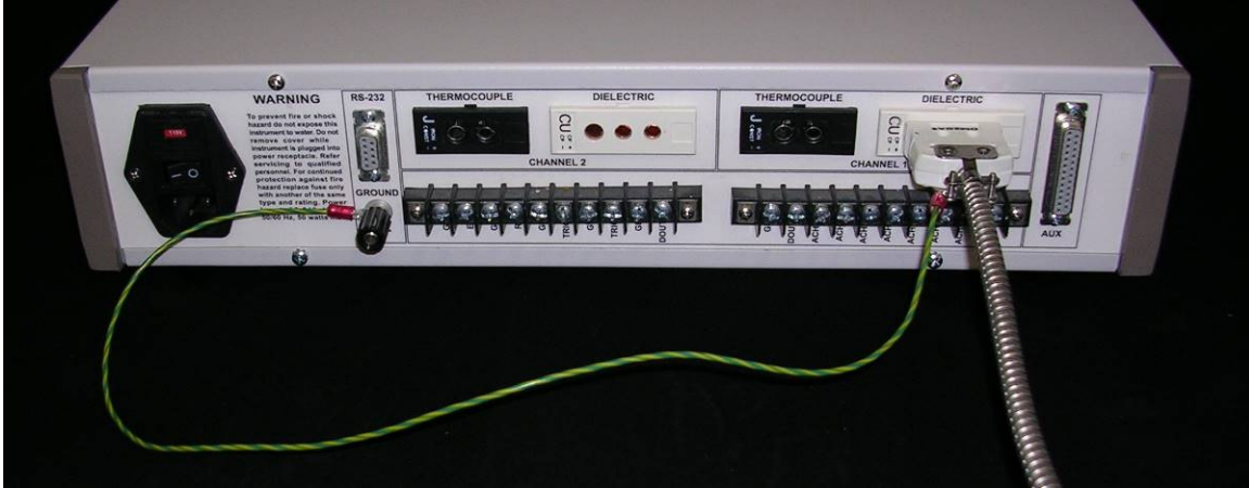
Figure 5 d Ground connection from LT-451 extension cable to LT-451 chassis
