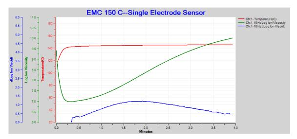
Figure 15-6 150 °C EMC cure data at 10 Hz
