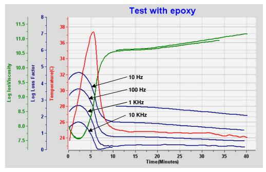
**Epoxy cure data after electrode polarization correction**
