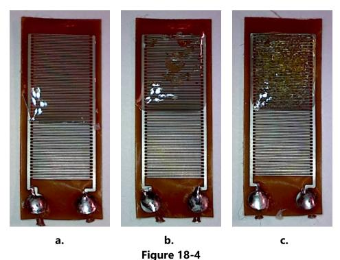
Correctly exposed (a), slightly (b) and significantly (c) over-exposed samples
