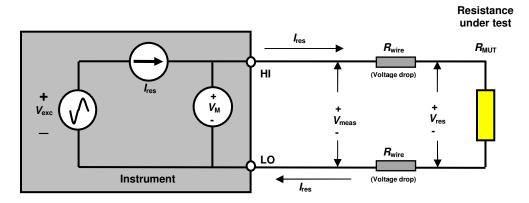
$V_{meas}$  = Voltage measured by instrument  $V_{res}$  = Voltage across resistor  $R_{MUT}$
