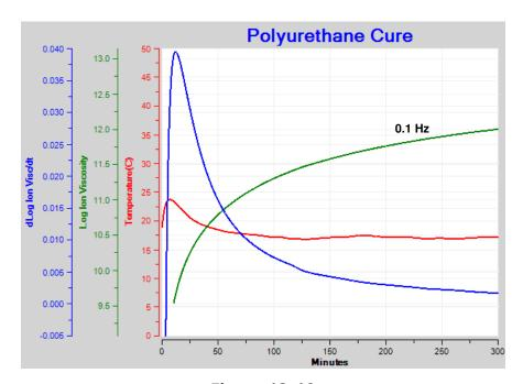
Figure 12-10 Ion viscosity and slope for curing polyurethane
