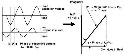
Raw measurement of  $I_{res}$  amplitude and phase allows calculation of G and C
