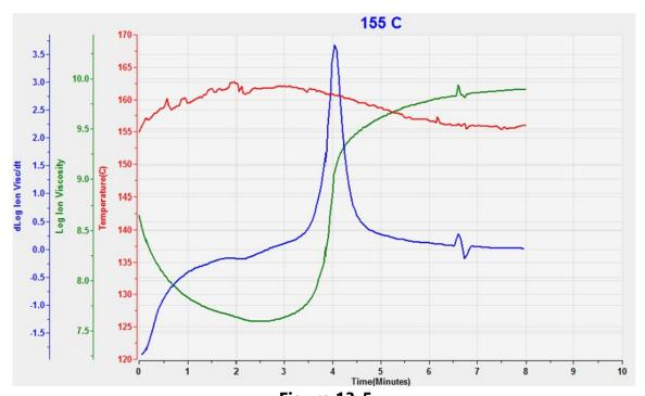
Figure 13-5 155 °C SMC cure data at 10 Hz
