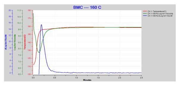
Figure 14-5 160 °C BMC cure data at 100 Hz
