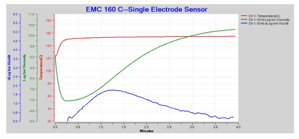
Figure 15-7 160 °C EMC cure data at 10 Hz
