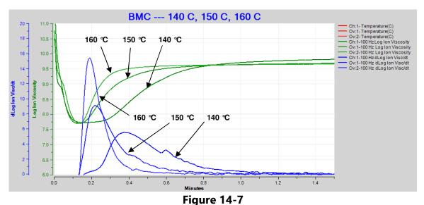
Overlay of 140 °C, 150 °C and 160 °C BMC cure data at 100 Hz
