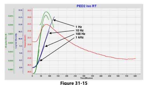
Ion viscosity and slope of ion viscosity for a vinyl ester cure Summary of Material Properties
