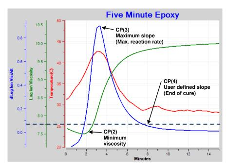
Figure 31-10 Ion viscosity and slope for 10 Hz frequency only
