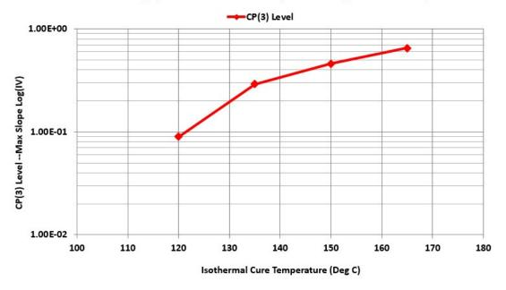
Figure 17-13 CP(3) level vs. cure temperature
