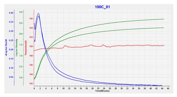
Figure 17-8 CFRP cure at 150 °C, 100 Hz and 1 kHz data
