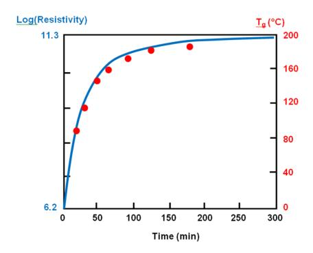
Figure 22-2  $T_{\rm g}$  and log(resistivity) vs. time during 200 °C isothermal epoxy cure<sup>3</sup>
