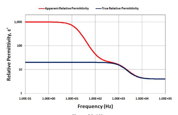
Figure 30-19b E' with electrode polarization and intermediate dipole time constant
