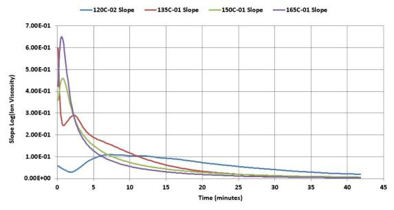
**Figure 17-11** Dependence of slope with isothermal cure temperature
