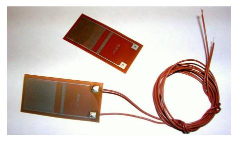
Figure 14-1 Mini-Varicon disposable sensor
