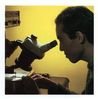
autoclave. The sensors communicate data to the system's computer about the chemical changes occurring. At left below, Micromet's Dr. Huan Lee is preparing a test of a polymer resin, dipping a ribbon sensor in the resin; the large black box is the Eumetric System II Microdielectrometer. Above, Lee is using a microscope to position the silicon microchip on the ribbon and at center right engineers are studying the results of the test.
