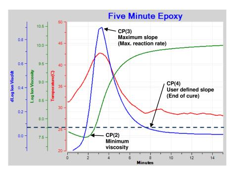
Figure 10-4 shows log(IV) from 10 Hz data as well as the resulting curve for slope.
