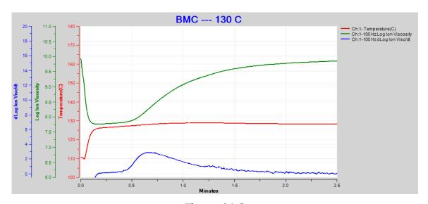
Figure 14-2 130 °C BMC cure data at 100 Hz
