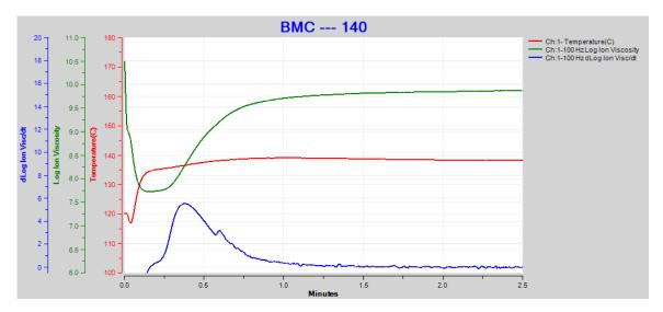
Figure 14-3 140 °C BMC cure data at 100 Hz
