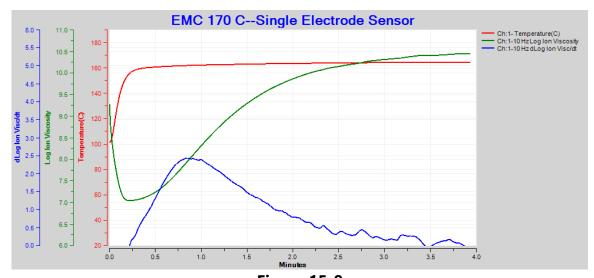
Figure 15-8 170 °C EMC cure data at 10 Hz
