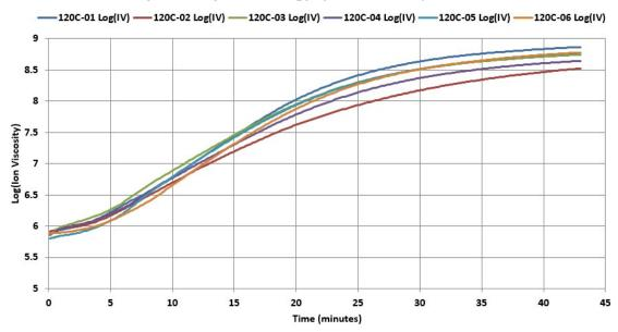
Figure 17-4 Log(*IV*) from cures at 120 °C of six samples of CFRP, 100 Hz data
