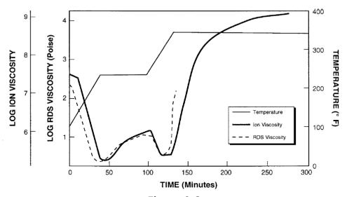
Figure 9-3 Ion viscosity for an epoxy resin cure with two ramp-and-hold steps<sup>2</sup>
