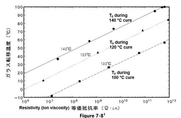
Glass transition temperature vs. resistivity (ion viscosity) for an epoxy
