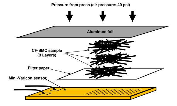
Figure 16-1 Lay-up of CF-SMC for tests
