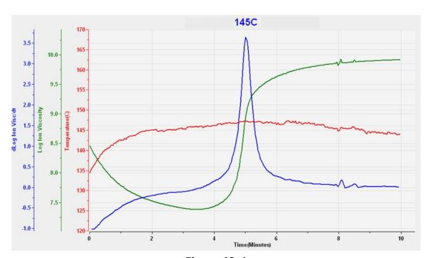
Figure 13-4 145 °C SMC cure data at 10 Hz
