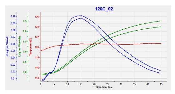
Figure 17-3 CFRP cure at 120 °C, 100 Hz and 1 kHz data
