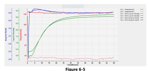
Cure of prepreg, two sensors simultaneously
