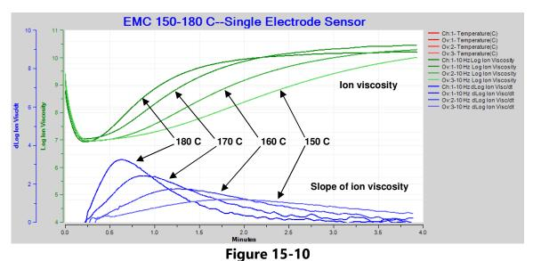
EMC ion viscosity (green) and slope (blue) at 10 Hz, cures at 150 °C, 160 °C, 170 °C and 180 °C
