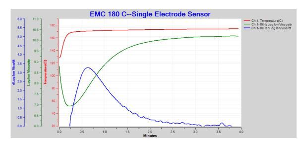
Figure 15-9 180 °C EMC cure data at 10 Hz
