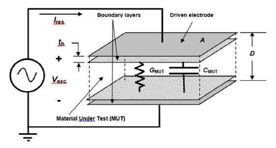
Figure 19-2 Electrical model of material on sensor with boundary layer
