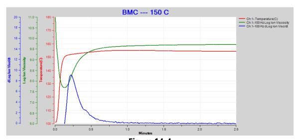
Figure 14-4 150 °C BMC cure data at 100 Hz
