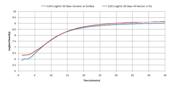
Figure 6-6 Log(*IV*) for Ceramicomb-1" and Mini-Varicon sensors
