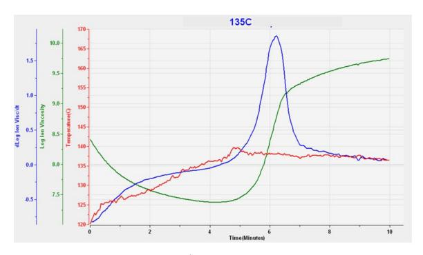
Figure 13-3 135 °C SMC cure data at 10 Hz
