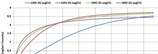
**Figure 17-10** Dependence of log(IV) with isothermal cure temperature
