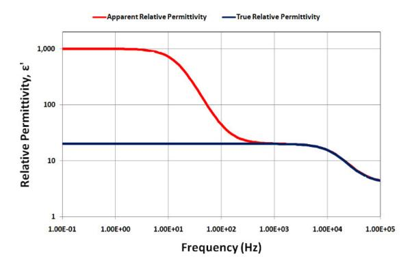
Figure 30-19a E' with electrode polarization and small dipole time constant
