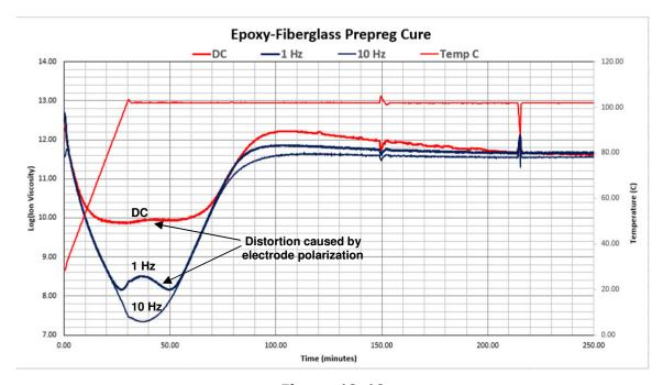
Figure 19-10 DC ,1 Hz and 10 Hz ion viscosity of epoxy-fiberglass prepreg cure
