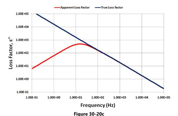
**E**" with electrode polarization and large dipole time constant
