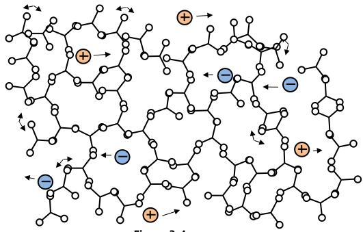
Figure 3-4 C-Stage resin (end of cure)
