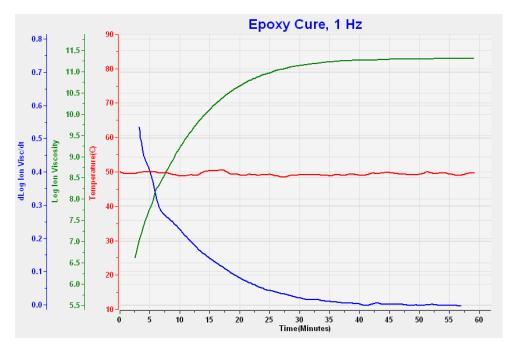
Figure 11-8 Isothermal epoxy cure at 50 °C
