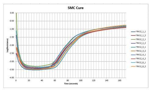
Figure 5-5 SMC resistance during cure, on a logarithmic scale
