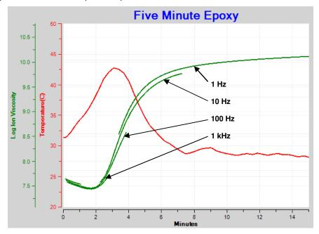
Figure 10-2 Ion viscosity—frequency independent resistivity only
