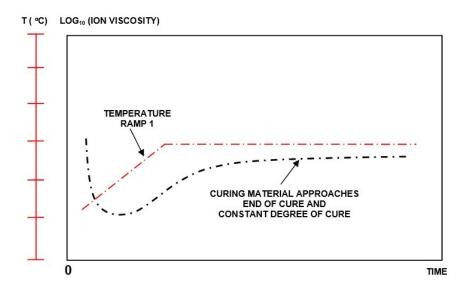
Figure 21-6 lon viscosity during cure
