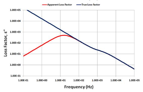
$\textbf{Figure 30-20b} \\ \textbf{$\epsilon''$} \ \ \textbf{with electrode polarization and intermediate dipole time constant}$
