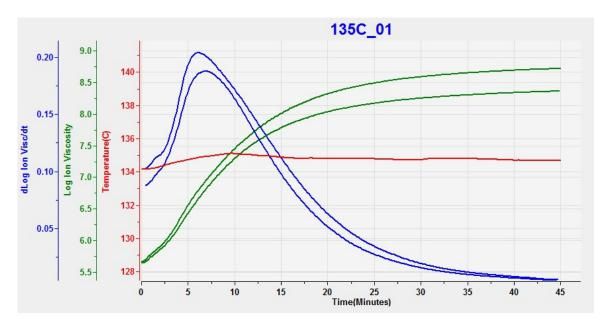
Figure 17-7 CFRP cure at 135 °C, 100 Hz and 1 kHz data
