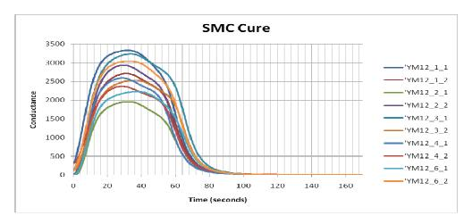
Figure 5-1 SMC conductance during cure, on a linear scale
