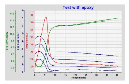
Multiple frequency loss factor and conversion to ion viscosity
