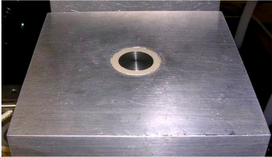
Figure 36-6 Unitrode-1" dielectric sensor in press platen
