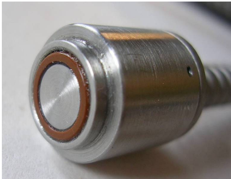
Figure 25-11 Dielectric sensor with single electrode
