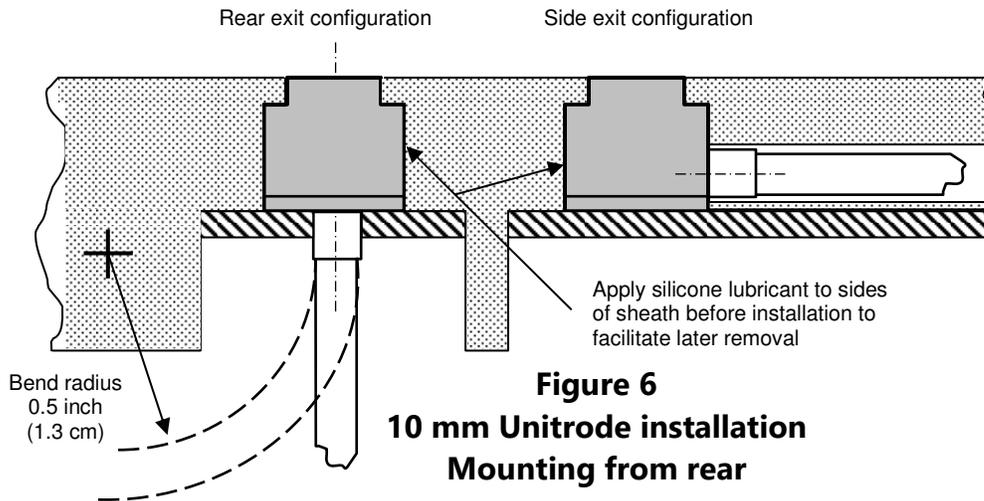
It is important to support the bottom plate of the sensor to prevent high pressures from pushing it out of position. To facilitate removal when necessary, silicone lubricant may be applied to the side of the sheath before installation.
